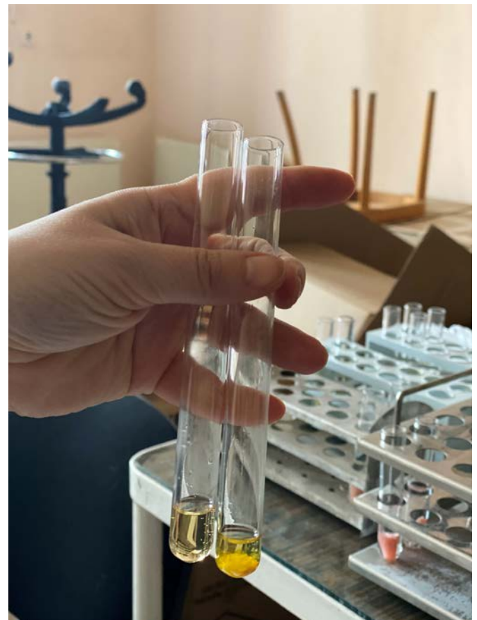
FIGURE 2. The immersion of samples in alcohol and gastric juice
